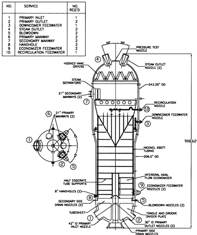
**Figure 1.** A typical PWR SG major components
