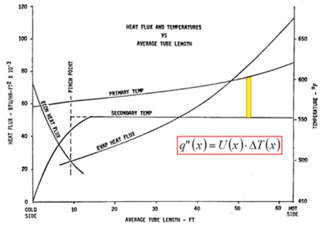
Figure 1 Heat flux and Temperature against Average Tube length
