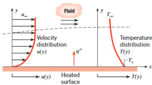
Figure 3. Boundary layer development in convection heat transfer
