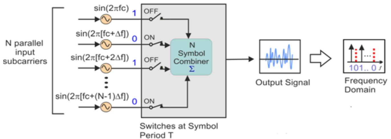
Figure 2. Simple OFDM Diagram
