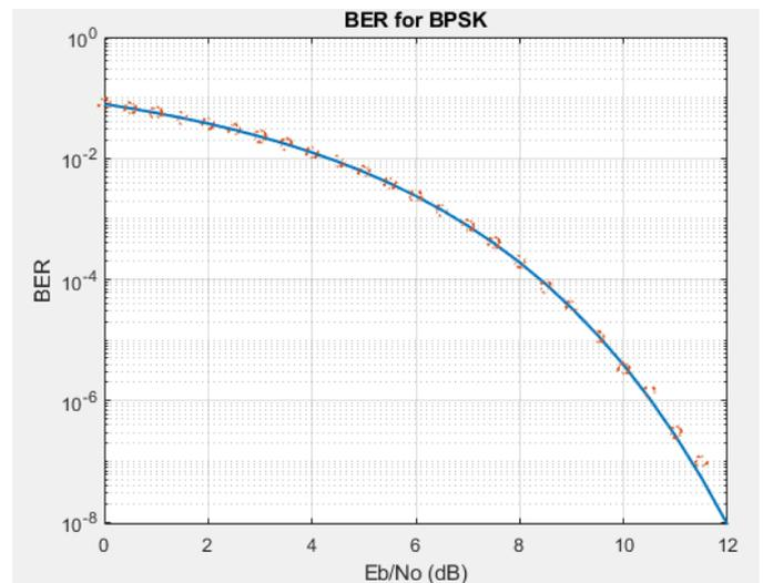
Figure 7. Bit Error Rate for BPSK
