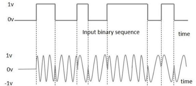
Figure 7. BPSK Modulated Wave
