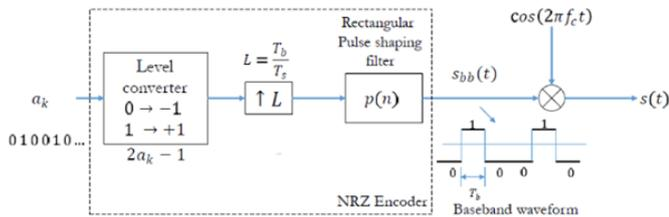
Figure 4. Transmitter section of BPSK
