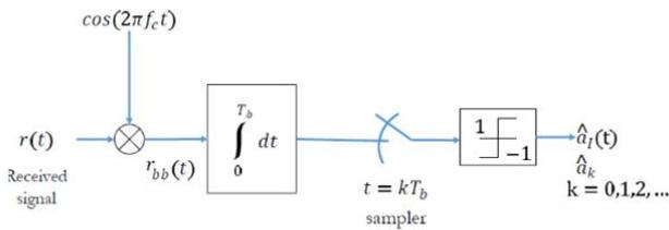
Figure 5. Receiver Section of BPSK.
