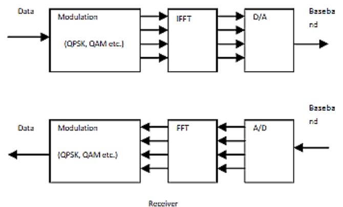
Figure 3. FFT OFDM Transmitter & Receiver
