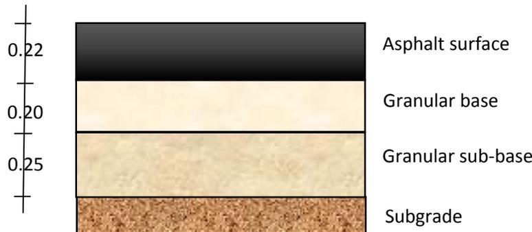
**Fig. 2.** Structural model for design
