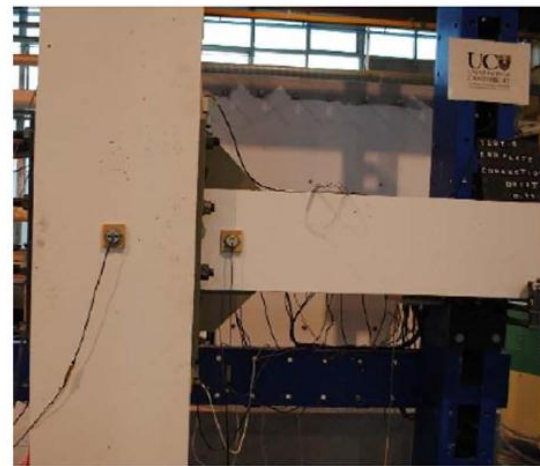
(a) Schematic layout of the connection (b) A sub-assembly with the end plate connection
