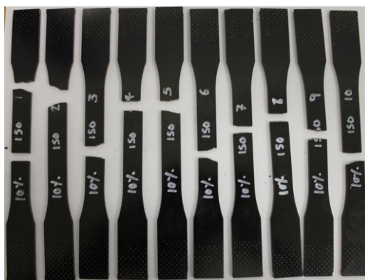
Figure 5: 10 weight percentage of 150 μm size CSP in epoxy resin composite specimens after tensile testing to failure
