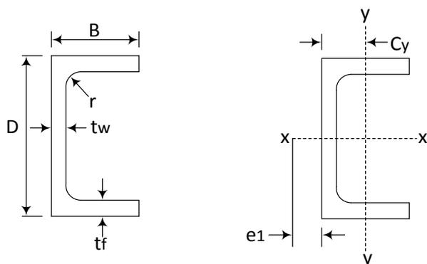
**Figure 1:** The aluminium channel cross-section representation
