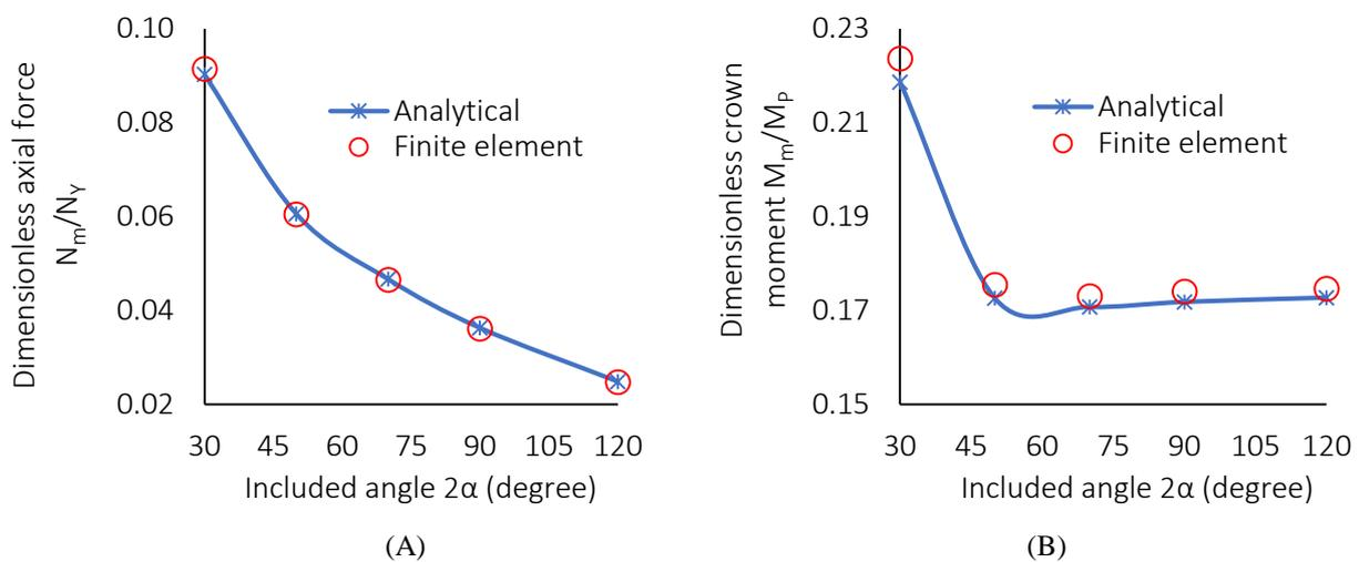
**Figure 4:** Comparison of the finite element and theoretical (A) axial compressive force and (B) bending moment at the crown at various included angles
