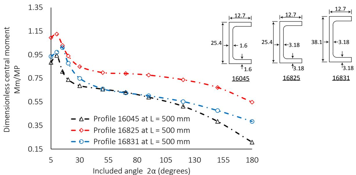
**Figure 7:** Cross-sections variations of the central bending moment with included angles
