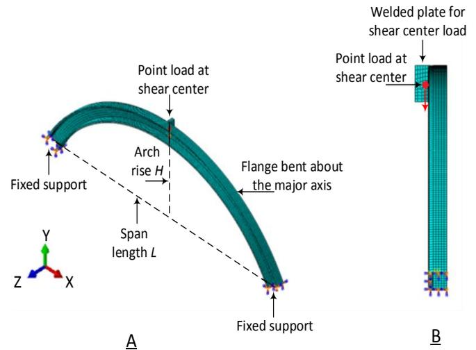
Figure 3: A sample of the finite element arch model (A) isometric view (B) side view B
