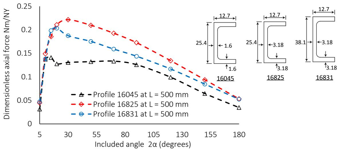
**Figure 5:** Cross-sections variations of the axial compressive force with included angles
