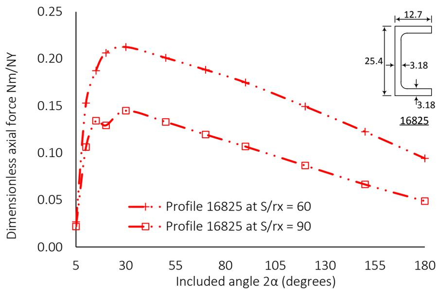
**Figure 6:** Slender ratios variations of the axial compressive force with included angles
