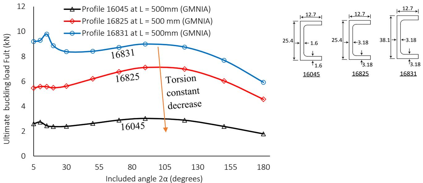
Figure 9: Cross-sectional effects on the inelastic lateral-torsional buckling load for fixed arches
