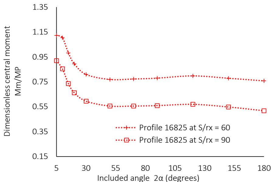
**Figure 8:** Slender ratios variations of the central bending moment with included angles
