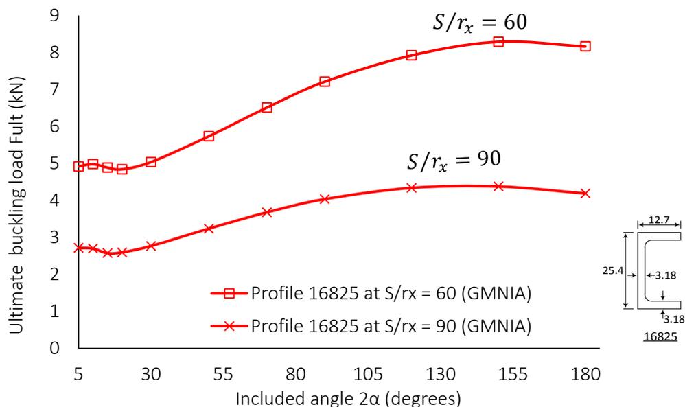
**Figure 10:** Slender ratios effects on the inelastic lateral-torsional buckling load for fixed arches
