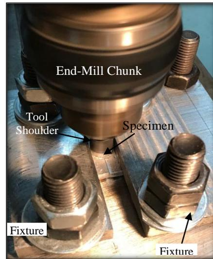
Fig. 2: Typical image of FSW process
