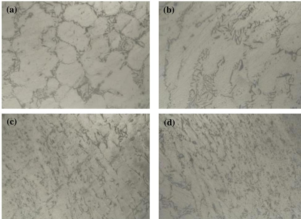
**Fig. 5:** Optical images of FSW of etched nanocomposite specimen, X200; a) Base metal: large and equiaxed grains, b) HAZ: large and elongated grains, c) TMAZ: small and elongated grains, and d) weld nugget, small and homogeneously distributed grains.
