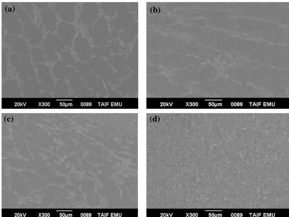
**Fig. 6:** SEM images of etched FSW of nanocomposite specimen, X300; a) Base metal, b) HAZ, c) TMAZ, and d) weld nugget
