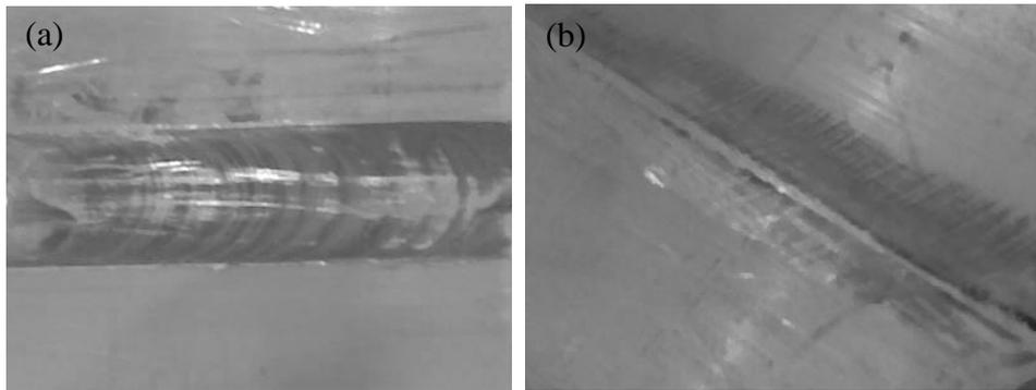
**Fig. 3:** Appearance of the as-weld nanocomposite sample; a) upper surface, and b) bottom face; welding conditions: weld speed, 1250 rpm and transverse speed, 30 mm/min.
