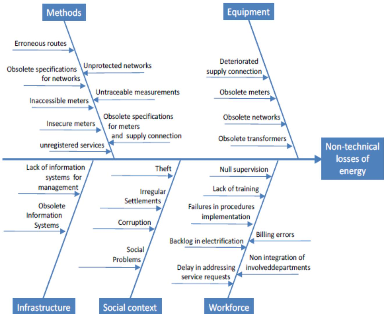
**Figure 3:** Causes of Non-Technical Losses in Distribution Systems
