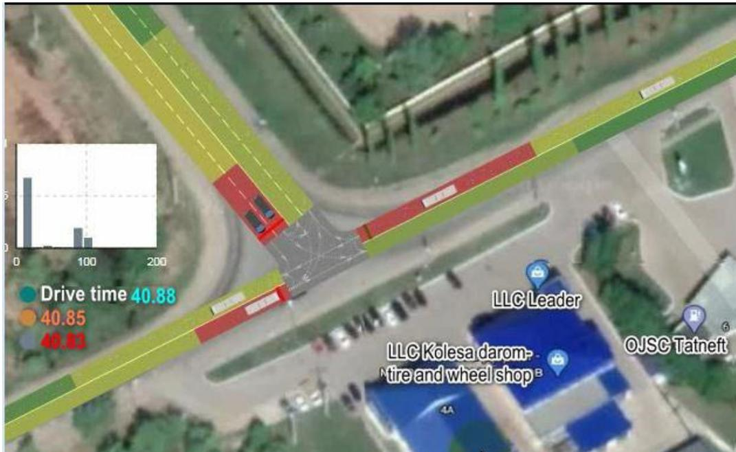
**Figure 4:** Results of running the intersection model with optimal parameters of the traffic light with a three-phase cycle
