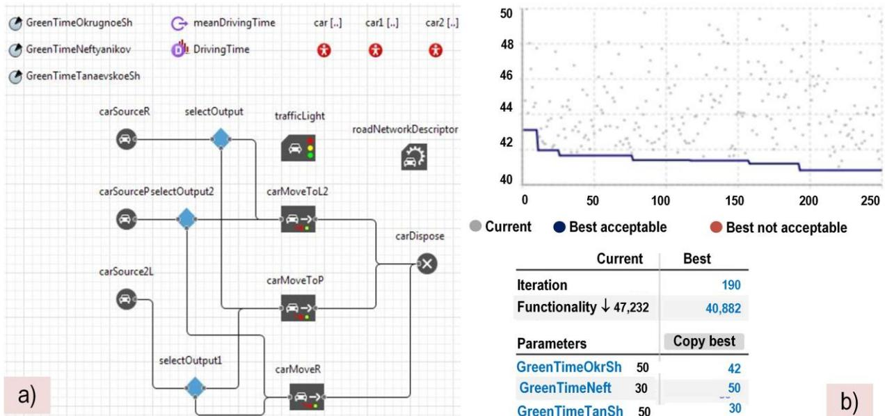
**Figure 3:** a) the structure of the IM crossroad of Elabuga; b) Results of the optimization experiment
