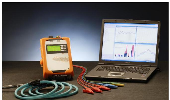
Fig. 1. A-EBERLE PQ BOX 100 used for the power audit
