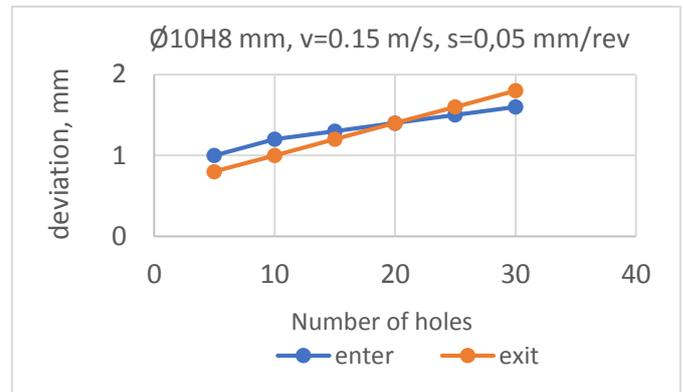
**Figure 5** - Effect of the number of drilled holes on the deviation. The degree of conformity of the diameters of the holes to the established tolerance was estimated by comparison. The target value corresponds to a rejection probability of 0.27%. To calculate the sigma level, we used the tolerance for the manufacture of holes adjusted by the tolerance for the manufacture of the tool and its wear. The adjusted tolerance  $\Delta_{dev}$  was 30 mkm.
