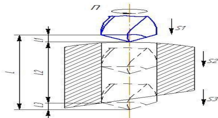
**Fig. 3.** Recommendations a method for drilling non-technological holes with variable feed.
