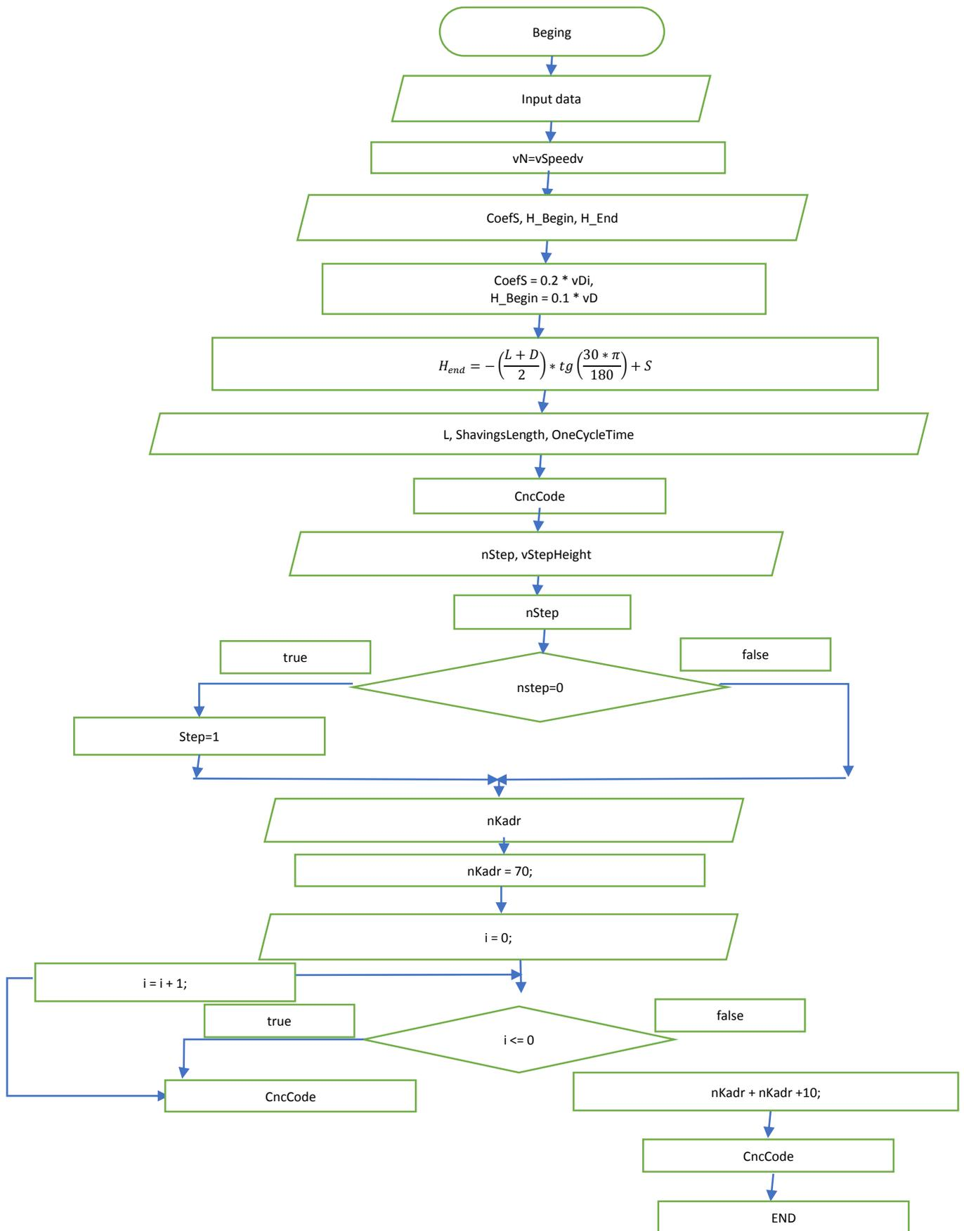
**Figure 4.** The block diagram of the method for producing chips with a predetermined length when drilling on machines with programmed control. [4]
