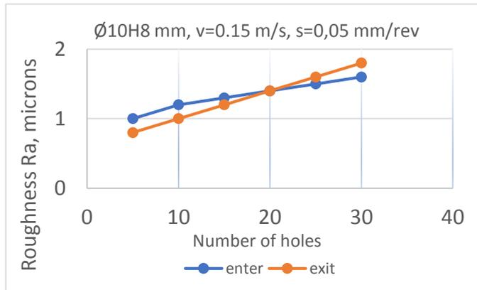
**Figure 6** - Effect of the number of drilled holes on the roughness
