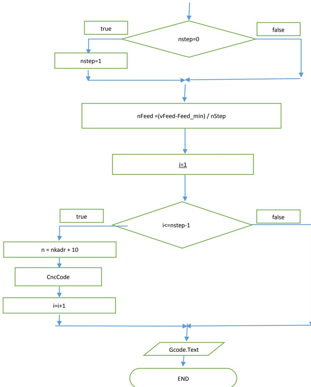
**Fig. 2.** Flow chart for drilling non-technological holes with variable feed.
