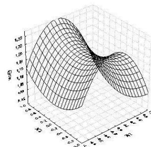
**Fig 3** Dependence of the strength of plywood when it is spalled over the adhesive layer after boiling for 1 hour
