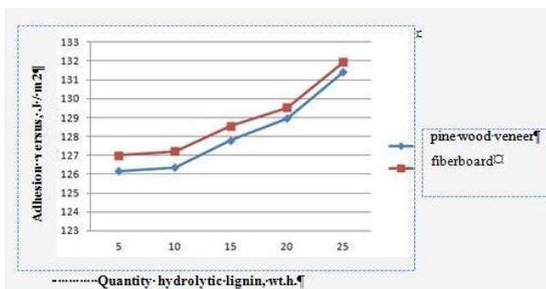
**Fig. 2.** Schedule of adhesion versus input quantity hydrolytic lignin in the adhesive composition
