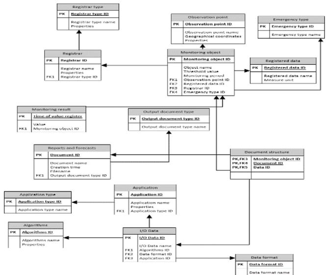
**Figure 6.** Database model of automated emergency situations monitoring and forecasting system in the Altai Republic
