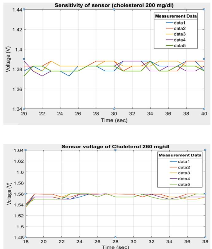
**Figure 5.** Sensor sensitivity on cholesterol measurement compared to invasive techniques
