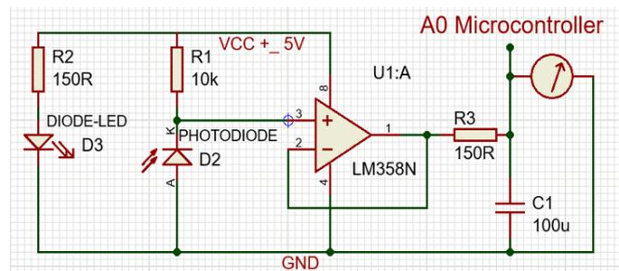
**Figure 3.** Schematic diagram of a cholesterol monitoring system
