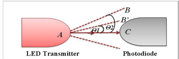
**Figure 1.** IR (LED) light reflection angle
