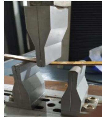
Fig. 5. Flexural Specimen Test of the BSRECM
