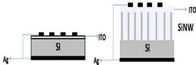
**Figure 2.** Schematic diagram Schottky solar cell with and without nanowires.
