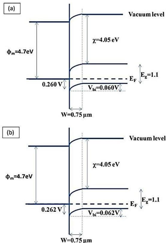
**Figure 3** Band energy diagrams (a) Si (b) Nanowires/Si substrates
