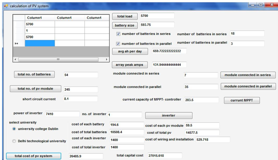
**Figure 6.** Conventional PV system of Delhi Technological University (number & cost)
