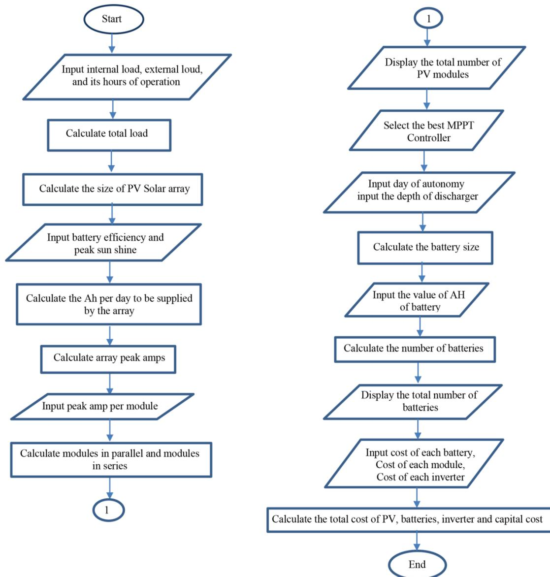
**Figure 8.** Flow chart represents the designing of the PV system.
