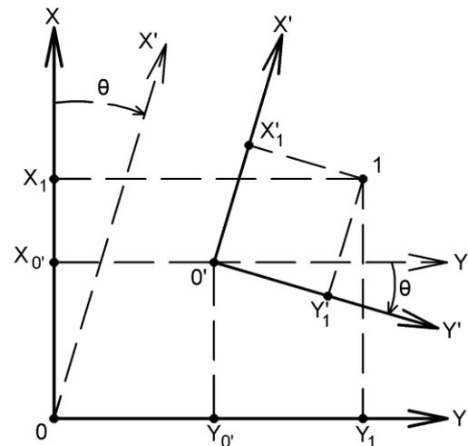
**Fig.1.** Elements for transforming one plane coordinate system into another.
