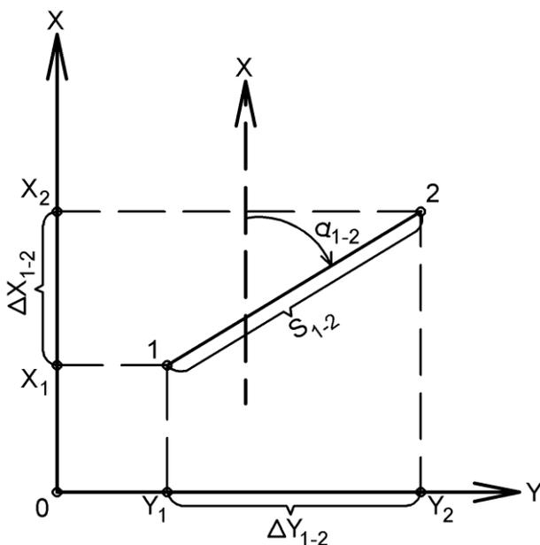
**Fig.2.** Elements of the forward and reverse geodetic task for calculation of parameters of the transition of one plane coordinate system into another.
