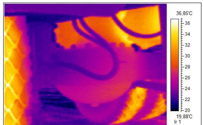
**Figure 1.** Thermal map of the intermediate axle in the KAMAZ vehicle
