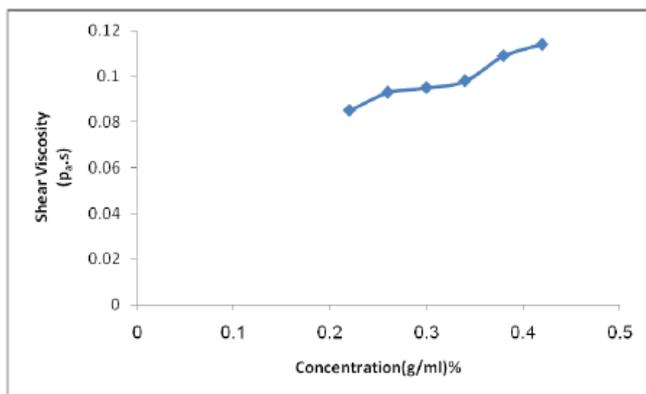
**Figure 2.** Shear viscosity change with concentration of PVA-CMC-PEG:
