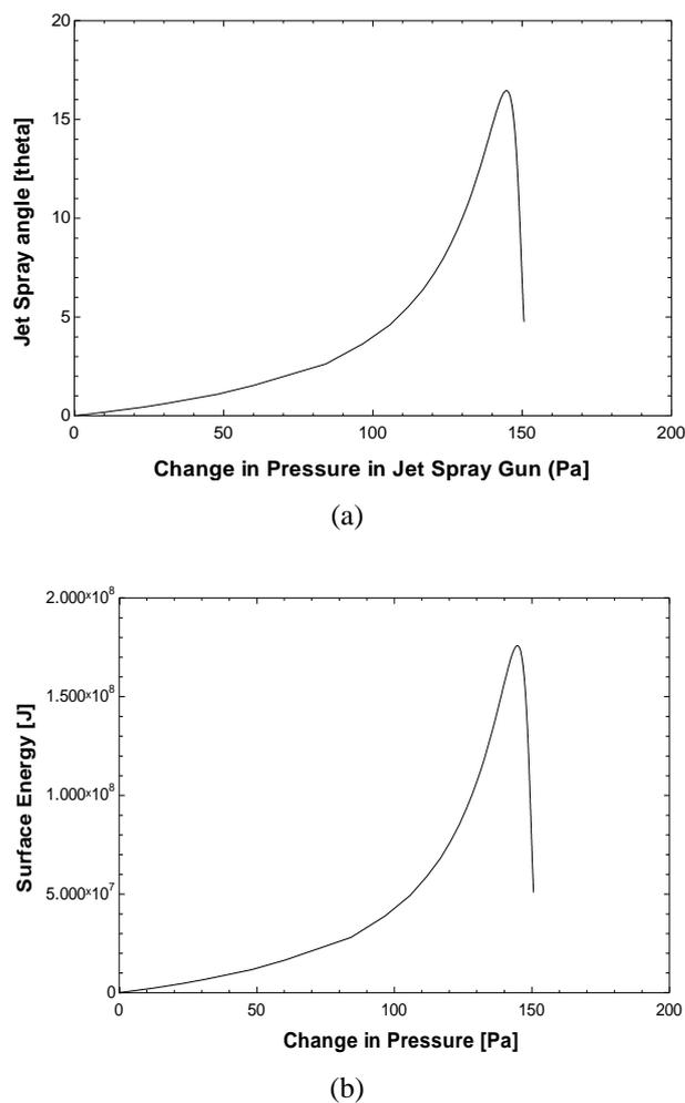
**Figure 4 (a)** Jet Spray angle during coating [theta] against change in pressure in jet spray gun during coating [Pa]
