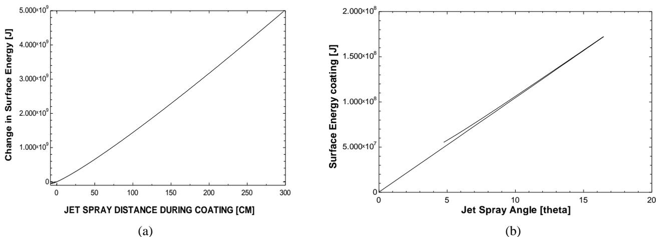
**Figure 3 (a)** Change in surface energy during jet spray coating [J] against Jet Spray Distance during coating process [cm]
