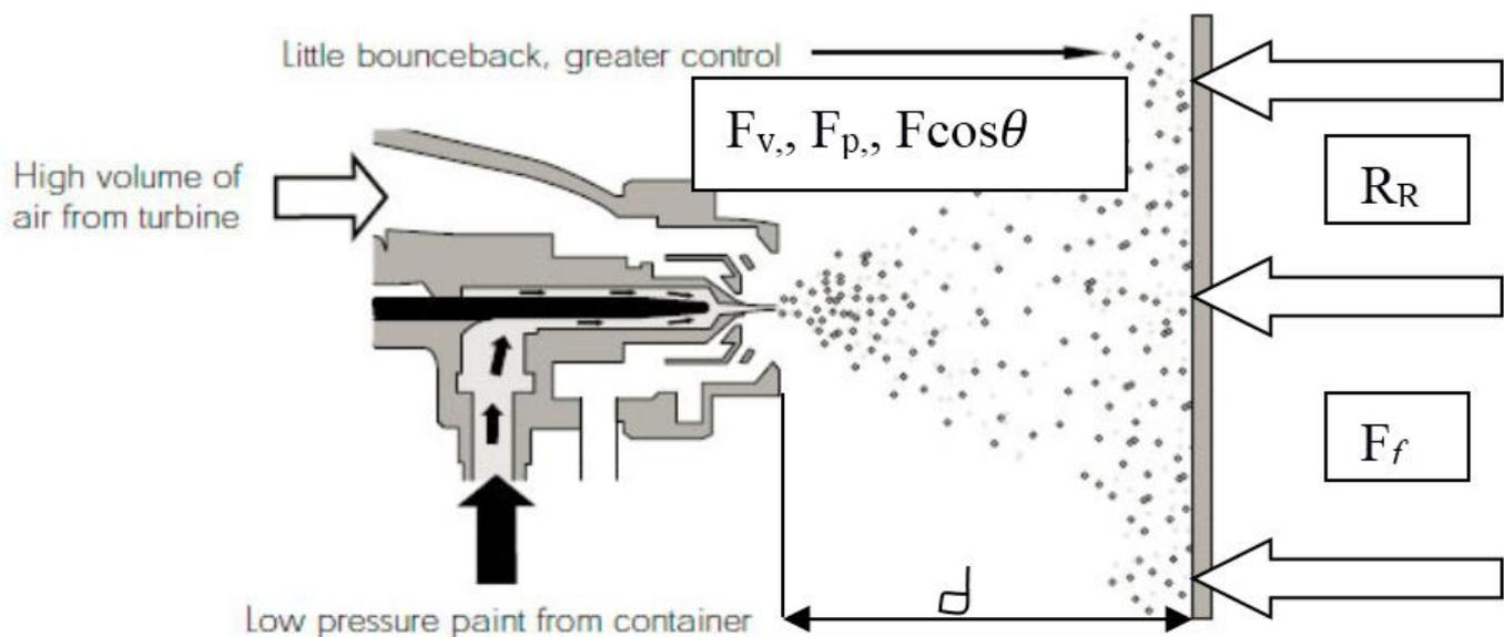
**Fig 1** Schematic diagram showing the main Forces during jet spray coating that impact nanoparticle scattering in a membrane.
