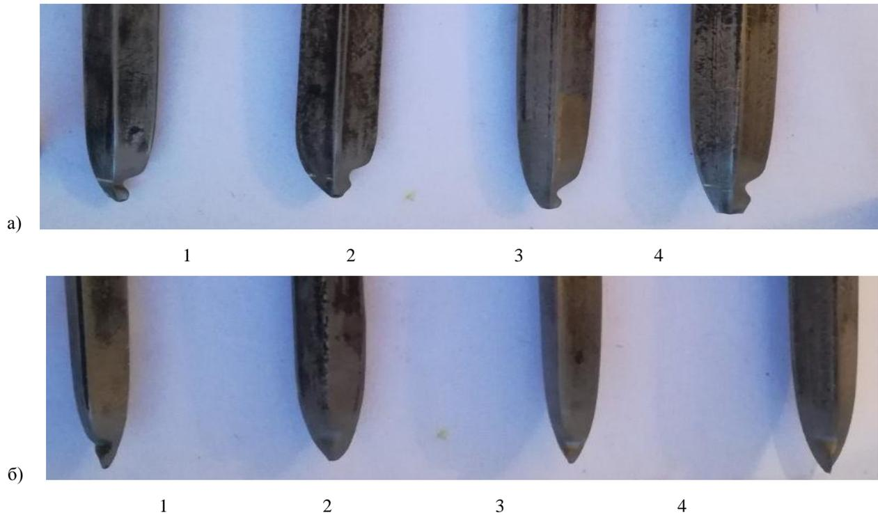
**Figure 4.** Overall view of tooth points wear after abrasive action according to the presented groups: a - side view; b - front view.
