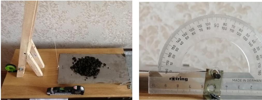
**Figure 4.** A laboratory installation for determining the angle of friction.
