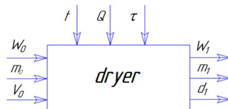
**Figure 1.** Block diagram of a drum dryer.
