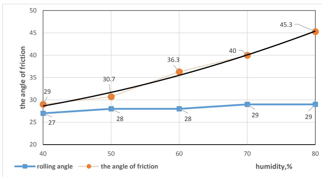
**Figure 5.** Dependences of the angle of friction of sapropel on humidity.
