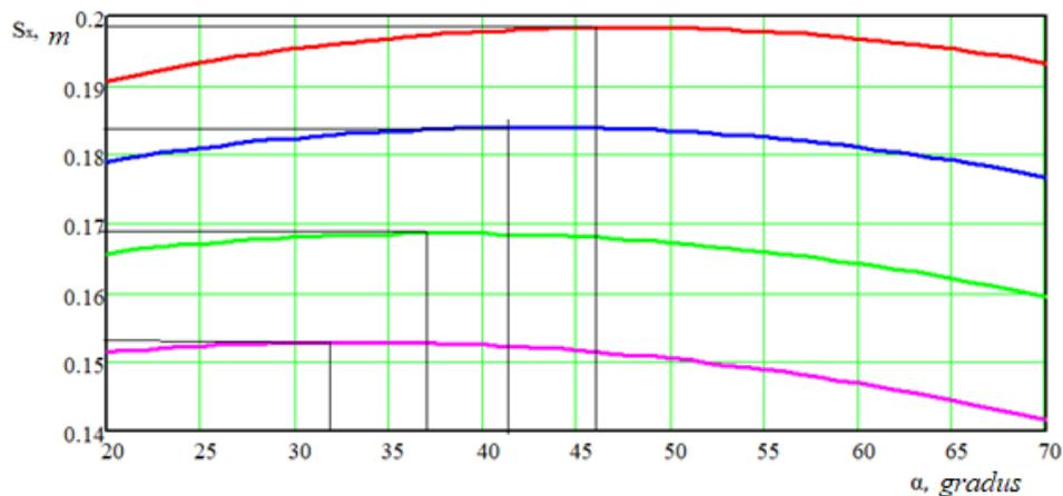
**Figure 8.** Dependence of the flight range of a sapropel particle on the initial angle of inclination of the blades.
