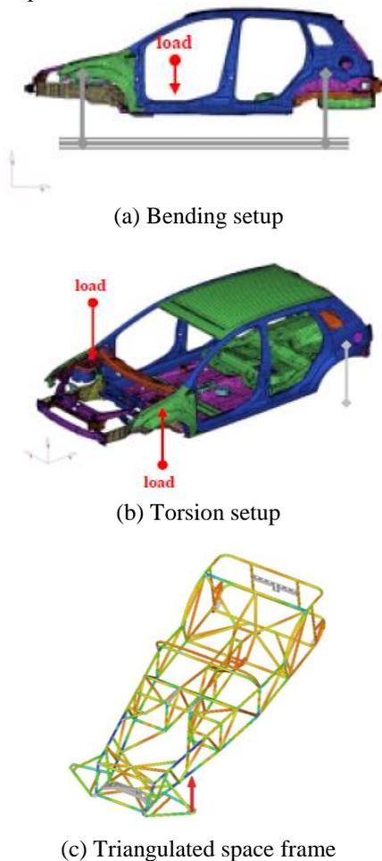
**Figure 10 FEM setup for stiffness modelling of integral body structures (a) bending and (b) torsion and (c) a triangulated space frame in torsion – courtesy (Magalhães & Agostinho, 2004; Barton & Fieldhouse, 2018)**
