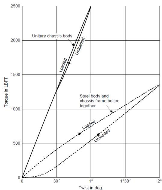
**Figure 5 Torsion stiffness tests comparison of steel unitary chassis and steel body and chassis bolted together car body structures of 1938 and 1939 models, respectively – courtesy (Swallow, 1939; Brown, et al., 2002)**
