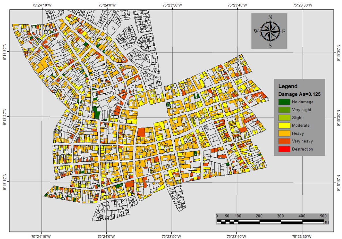
**Fig. 8.** Damage scenarios for  $A_a = 0.125$ . Design earthquake
