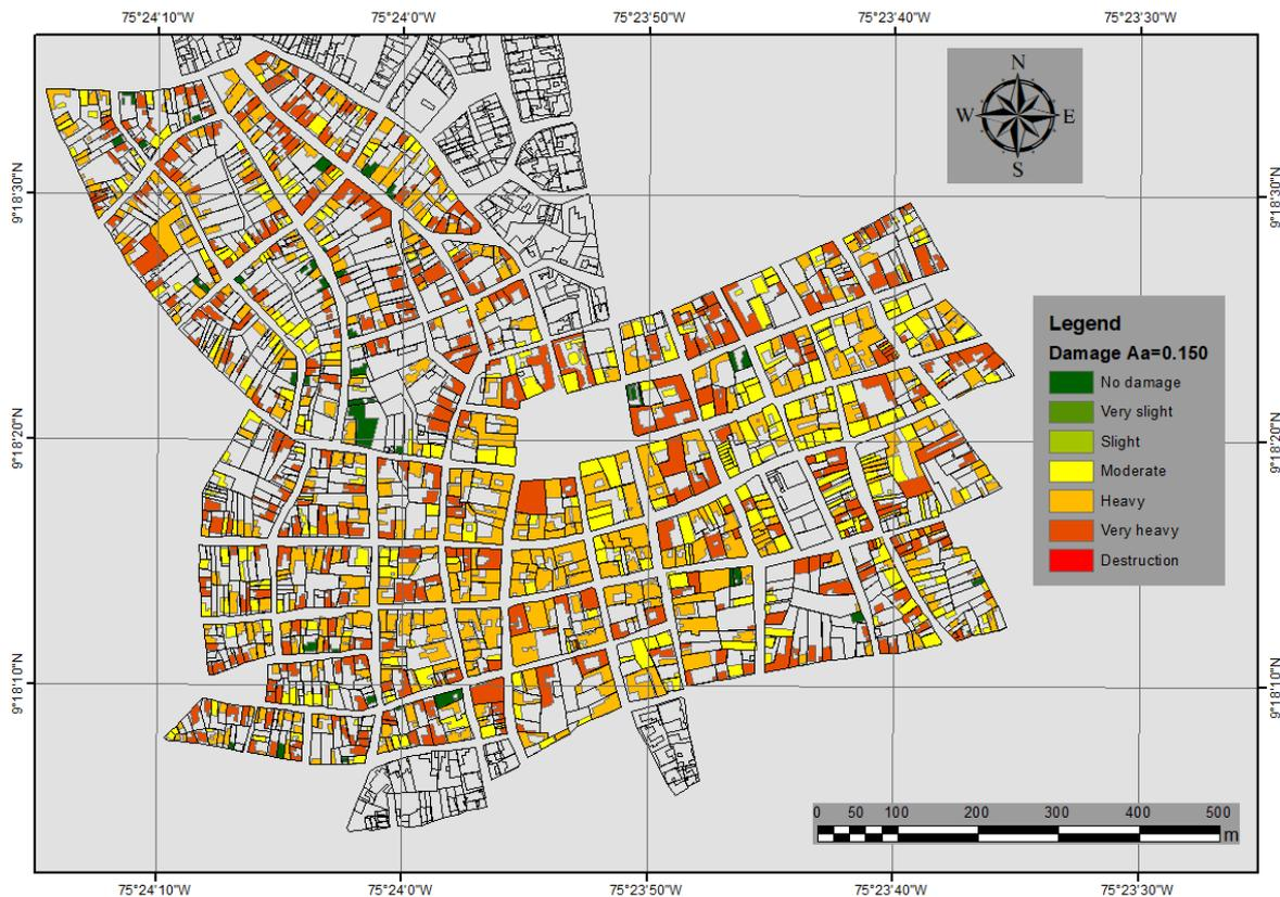
**Fig. 9.** Damage scenarios for  $A_a = 0.15$ . Severe earthquake
