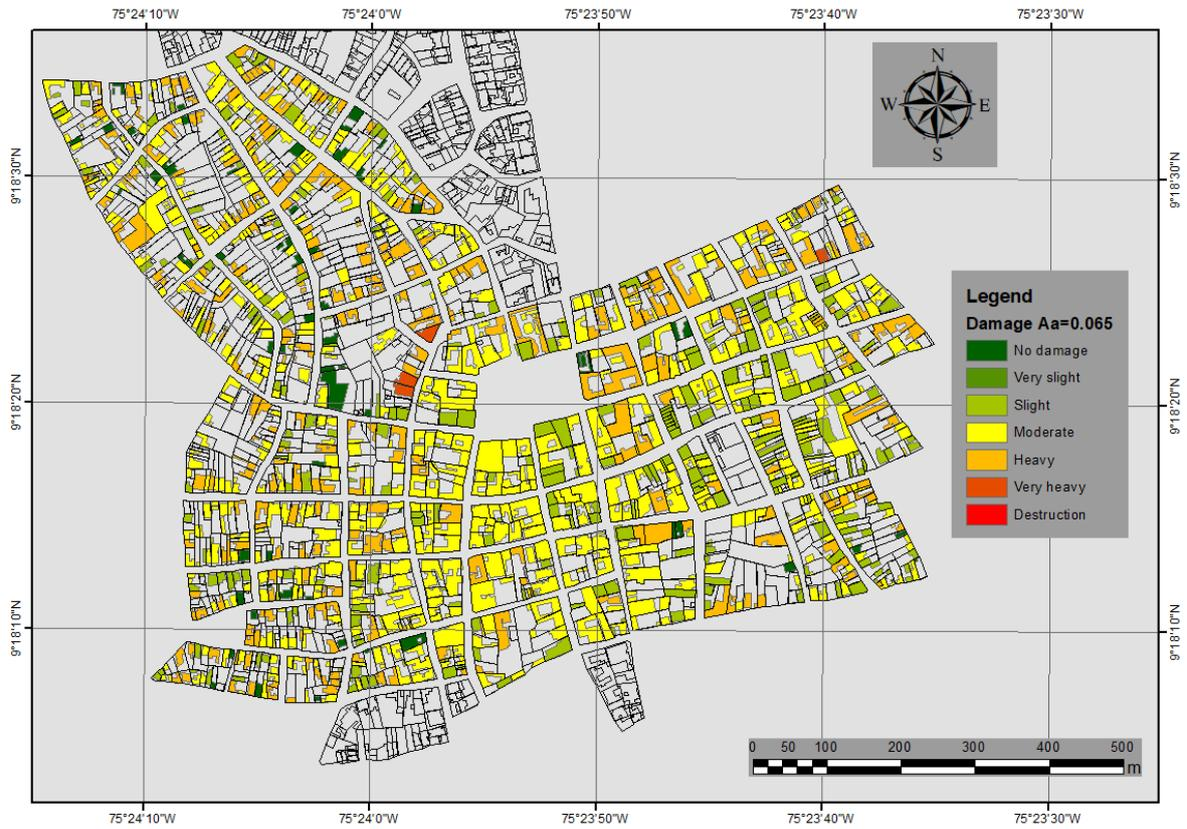
**Fig. 7.** Damage scenarios for  $A_a = 0.065$ . Service earthquake
