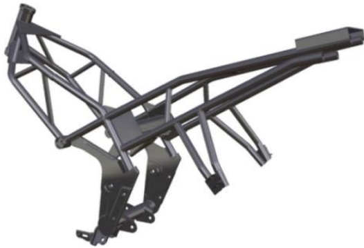
Fig. 4. The initial 3D solid model of a new motorcycle frame
