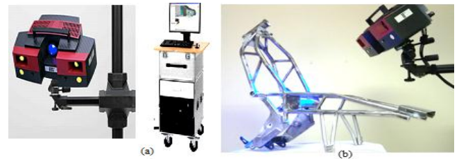
Fig. 2. (a) 3D Scan GOM Atos Triple Scan II; (b) Scanning of the prototype
