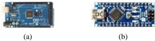
**Figure 3.** Microcontrollers: (a) Arduino Mega.; (b) Arduino Nano.
