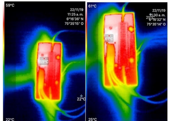
Fig. 9. Minimum and maximum levels achieved with a current of 1A and a heatsink with ventilation
