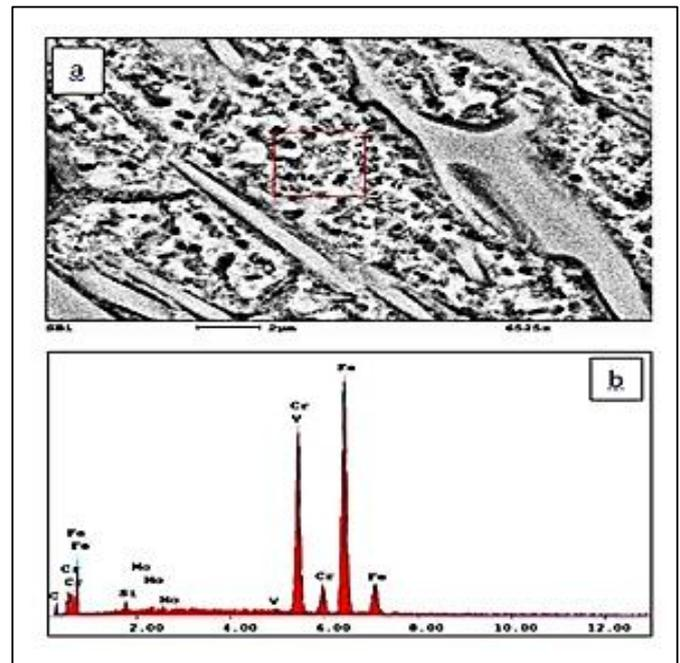
**Figure 3:** (a) SEM micrographs show secondary carbides in martensitic matrix and (c) EDS analysis of the matrix.
