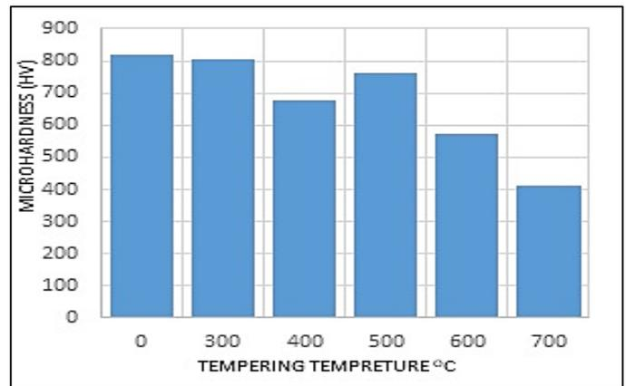
**Figure 6:** The influence of tempering temperature on the microhardness of air hardened alloy at 950°C
