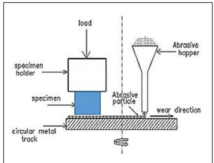
**Figure 1:** Schematic representation of the three body abrasion test (loaded specimen against rotating steel wheel).
