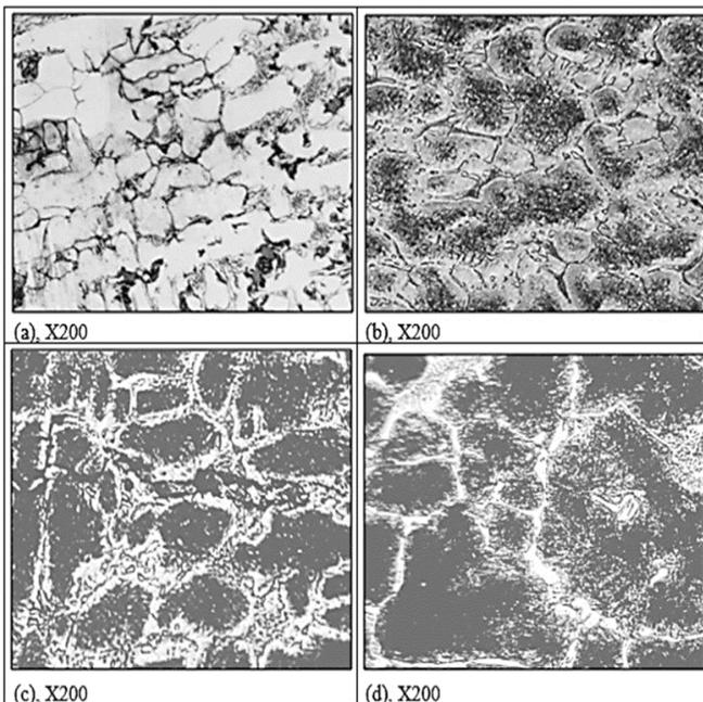
**Figure. 2:** Optical micrographs show the different microstructures of alloyed cast iron in as-cast and heat treated conditions; (a) as-cast, (b) austenitized at 900°C, (c) austenitized at 950°C, and (d) austenitized at 1000°C, followed by air cooling.
