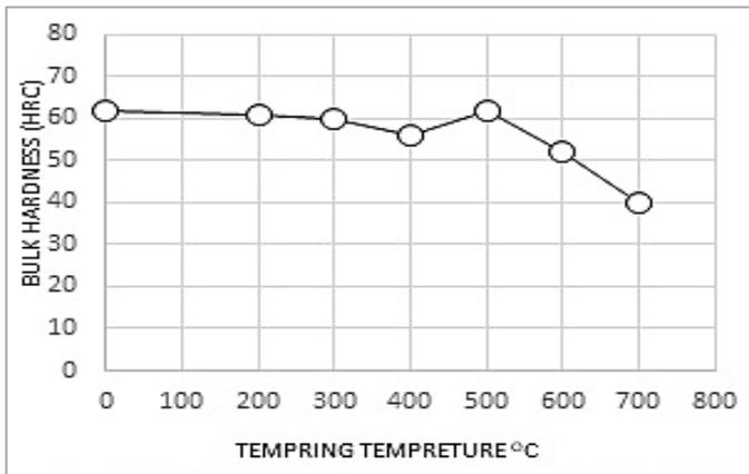
**Figure 8:** The effect of tempering temperature on the bulk hardness of the investigated alloy
