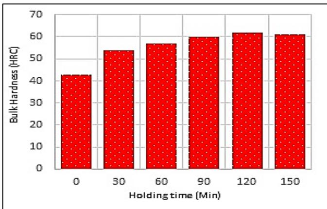
**Figure 5:** The effect of holding time on the bulk hardness of the investigated alloy at 950°C.
