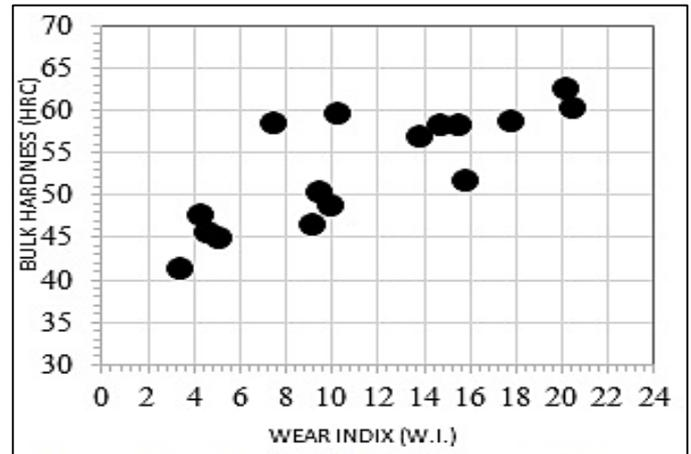
**Figure 9:** The relationship between matrix bulk hardness and abrasion resistance of the investigated alloy at different conditions.
