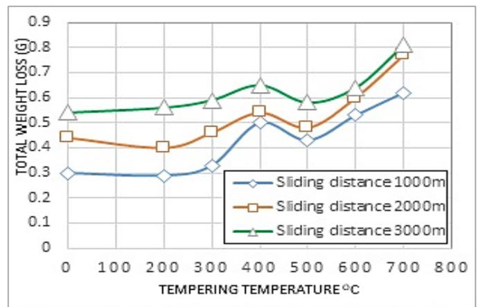
**Figure 7:** The influence of tempering temperature on the abrasive weight loss (g) of the investigated alloy at different sliding distances of 1000, 2000, and 3000m.
