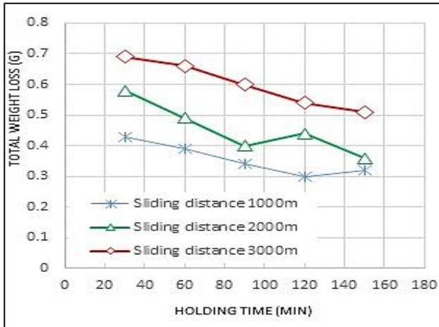
**Figure 4:** The influence of holding time on the abrasive weight loss (g) at different sliding distances 1000, 2000, and 3000m at 950°C.
