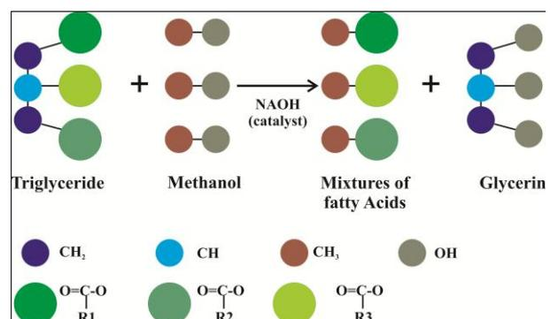
Figure 1. Transesterification Reaction
