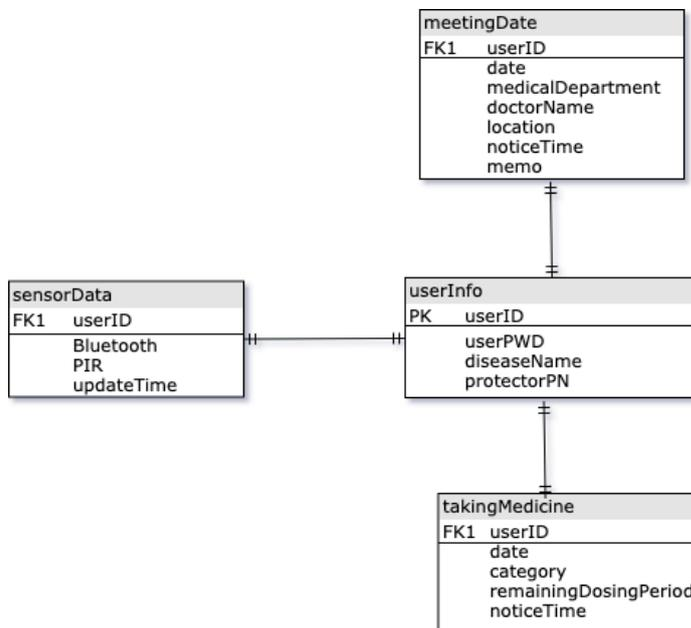
Fig. 3. Schema of the reminder system
