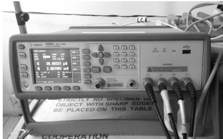
Fig. 1: LCR meter used for damage detection.
