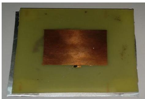
Figure 9: Photograph of fabricated antenna
