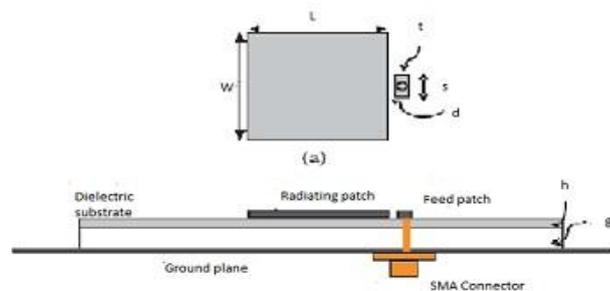
**Figure2:** Basic geometry of capacitive fed Microstrip antenna
