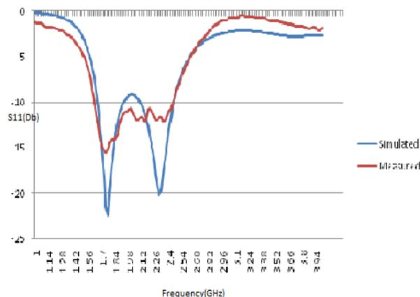
Figure 10: S11 of Measured and Simulated Microstrip antenna
