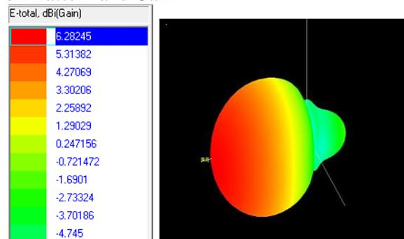
Figure 8: 3D Pattern and gain of Microstrip antenna
