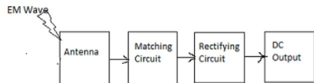
**Figure 1:** Block diagram of RF energy harvesting system
