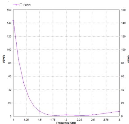
Figure 5: VSWR plot of Microstrip antenna
