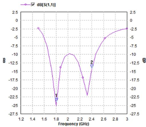
Figure 4: Simulated S11(dB) Vs Frequency (Ghz)
