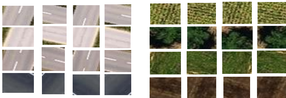
Figure 4. Examples of boxes used for training-positive boxes, asphaltic road and negative boxes.
